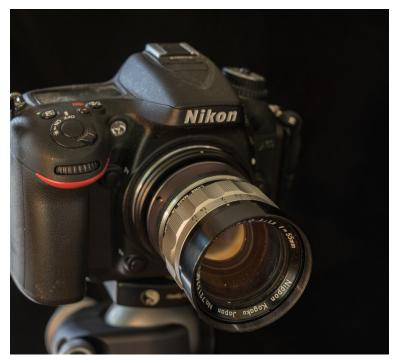
Lens: Nikkor "O" 55mm, f/1.2 CRT Oscilloscope
